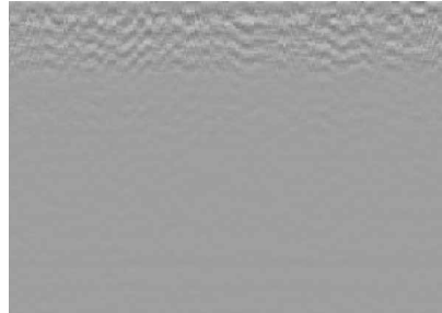
Clean Skyshot: minimal background noise/EMI is visible.
